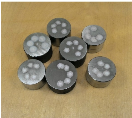
Spark spots on burning samples
